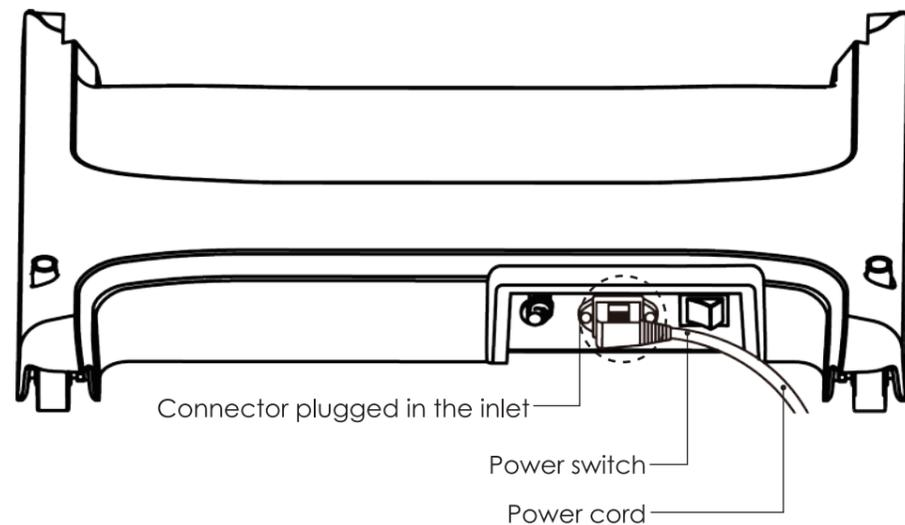
4 After installation is completed, insert the power plug into the power outlet. Turn on the power switch and press ON/OFF button on the remote controller to start select the massage functions.
