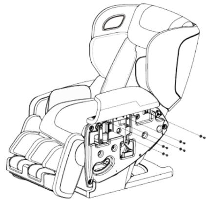
2 Fasten the arm unit with flat washer  $\varnothing 8.2 \times \varnothing 18.0 \times 1.4T$  and round-head hexagonal socket screw  $M8 \times 1.25P \times 10L$  firmly in five positions.
